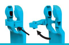
b. Position the drip chamber appropriately. Note the correct positioning of different types of drip
